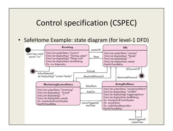
The diagram indicates how the system responds to events as it traverses the four states defined at this level.
