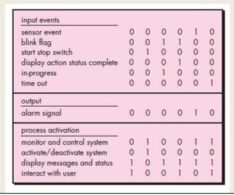
The PAT represents information contained in the state diagram in the context of processes (transformations), not states. That is, the table indicates which processes (bubbles) in the flow model will be invoked when an event occurs
