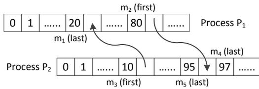
**Figure 2: Inter-process impact constrained by message passing.**
