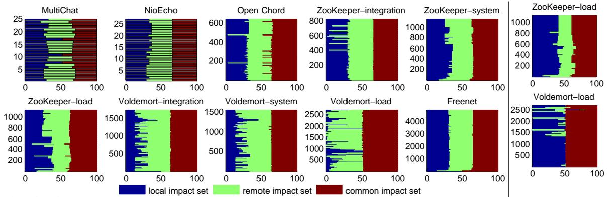
**Figure 6:** Left to l: composition of impact sets given by the basic DISTIA for all queries ( $y$  axes) expressed as the percentages ( $x$  axes) of local, remote, and common impact sets in the whole impact set per query, for each subject and input type (atop each plot as the title). Right to l: composition of impact sets given by the enhanced DISTIA for two subjects/inputs with the best effectiveness gains.
